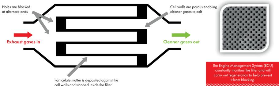
Because fuel and air do not mix as thoroughly in diesel engines as they do in petrol engines, fuel-dense pockets produce soot when ignited. This soot is the by-product of incomplete combustion.
