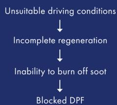
Other causes of a blocked DPF can be ash build-up or defects elsewhere within the engine. Replacing a blocked DPF without correct diagnosis of the genuine fault will only cause the new DPF to also become blocked!
